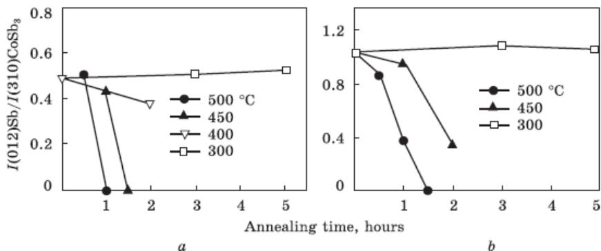
Fig. 5. Dependence of the intensity ratio of the  $I(012)Sb/I(310)CoSb_3$  diffraction peaks for  $CoSb_{3.6}$  (a) and  $CoSb_{4.2}$  (b) films on the annealing time in vacuum within the temperature range of 300–500 °C
