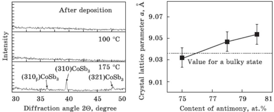
Fig. 1. X-ray patterns of as-deposited CoSb<sub>3.5</sub> film on substrate at a room temperature and after heating ( $\lambda K\alpha\beta$ -Fe)
