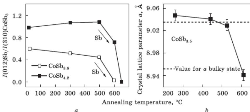
Fig. 4. Influence of annealing temperature for  $\text{CoSb}_{3.6}$  and  $\text{CoSb}_{4.2}$  films (in vacuum) on the change of (a) ratio of intensities  $I(012)\text{Sb}/I(310)\text{CoSb}_3$  of diffraction reflections and (b) the lattice parameter  $a$  for  $\text{CoSb}_3$  phase
