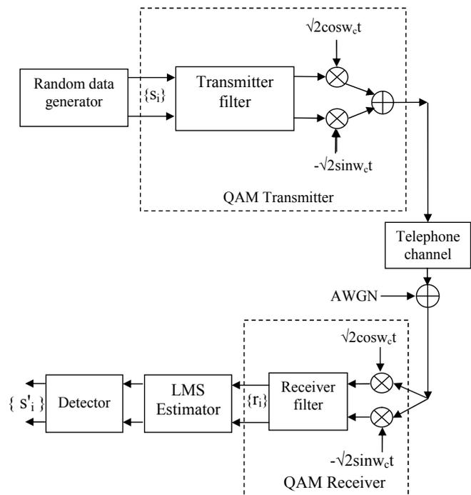
Fig. 1. Model of data transmission system
