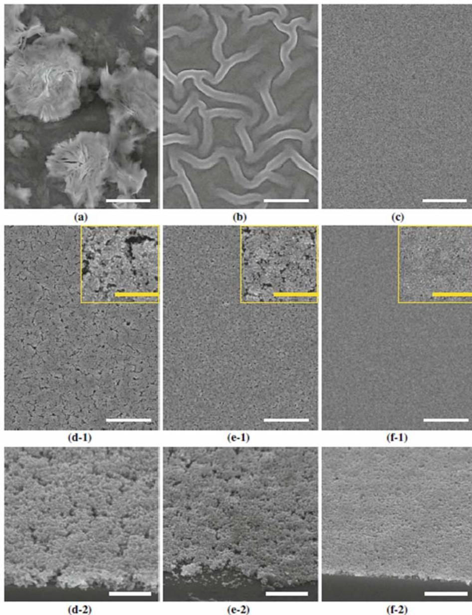
**Fig.5. SEM images of seed layers prepared on the hot plate at a 100°C, b 150°C, c 250°C, and those prepared at 100°C in a petri dish from precursors d 1.2 M ZnAc, e 0.5 M ZnAc, and f 0.5 M ZnAcH. The bars are 2  $\mu\text{m}$ , and the bars in the expanded image are 400 nm. d-2, e-2, and f-2 show the 40° images from upper side [15]**
