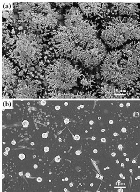
**Fig. 1. A set of SEM micrographs showing the dendritic character of morphological features of the ZnO thin film grown on Si substrate by sol-gel spin process using zinc nitrate as the precursor material [9]**
