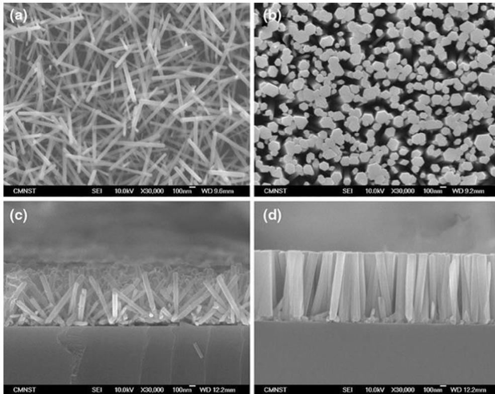
**Fig. 4** FE-SEM images of ZnO nanowires synthesized on a Si substrate coated with ZnO seedlayer films. The ZnO films were prepared by the sol-gel method with different sol concentrations a 0.05 M, plan view b 1.0 M, plan view c 0.05 M, crosssection view d 1.0 M, crosssection view [10]
