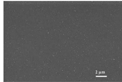
**Fig. 2. SEM micrograph showing the smooth character of morphological features of the ZnO thin film grown on Si substrate by sol-gel spin process using zinc acetate as the precursor material [9]**
