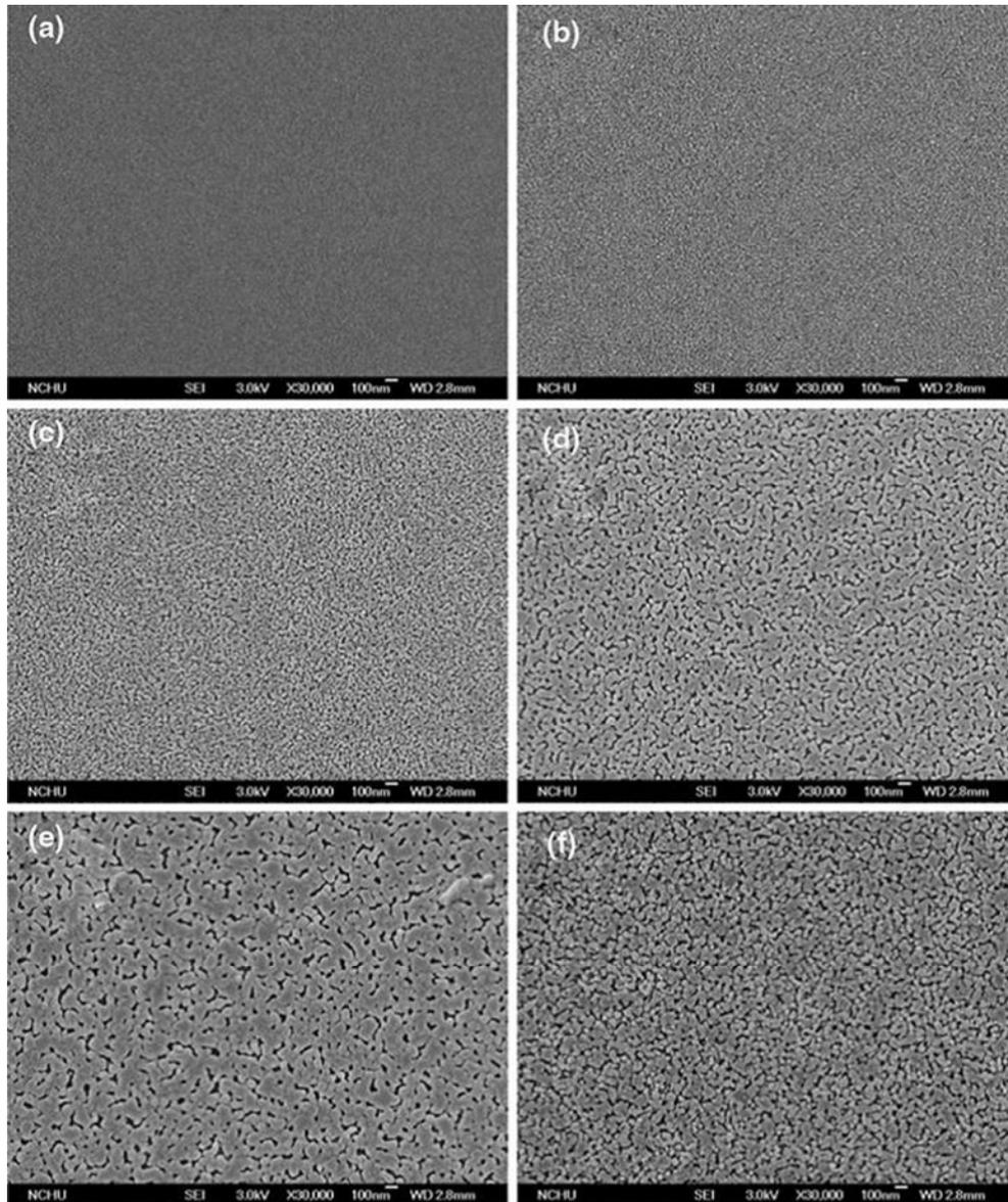
**Fig. 3. FE-SEM plan-view images of ZnO seed-layer films prepared with different sol concentrations a 0.05 M, b 0.1 M, c 0.3 M, d 0.5 M, e 1.0 M, f 1.2 M [10]**
