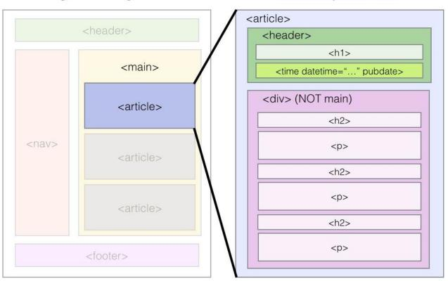
Fig. 1.10. Structure HTML5 sectioning element [6]
