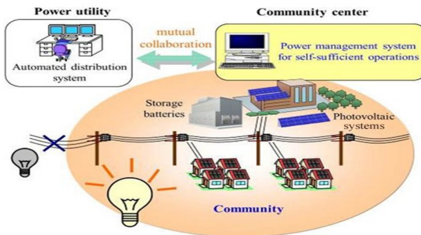
Electric Power Management System for Self-sufficient Operation
