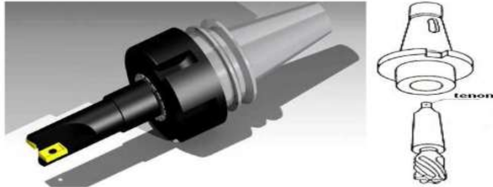
Fig.7. Mounting Tool on Tool holder
