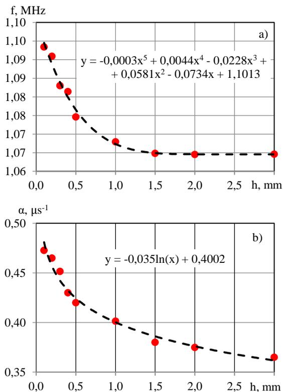
Fig. 7. The dependence of the values of ECP signal natural frequency (a) and ECP signal attenuation (b)
