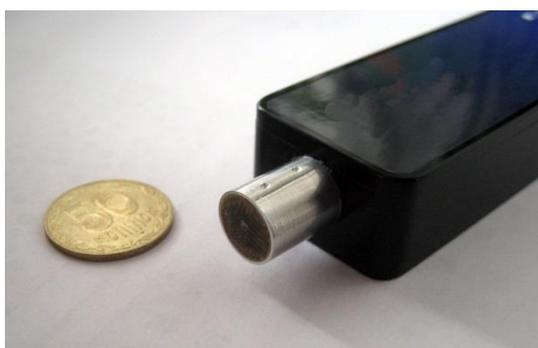
Fig. 3. The transducing unit of the ECNDT system
