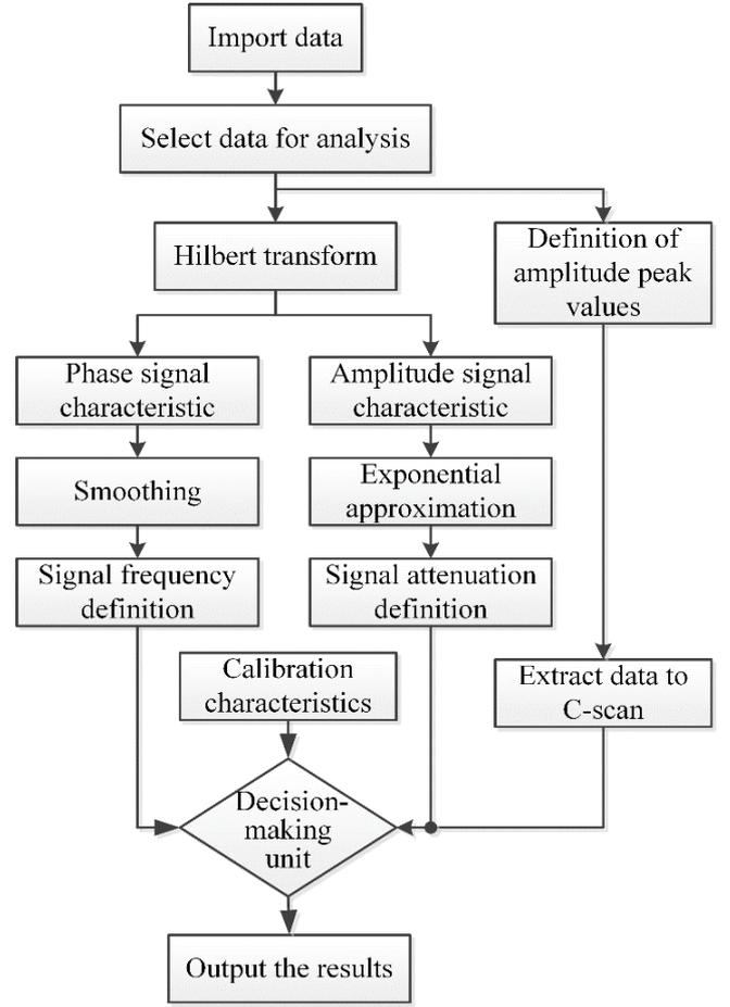
Fig. 1. Methodology of ECP signal processing
