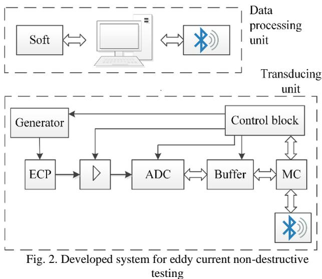
Fig. 2. Developed system for eddy current non-destructive testing
