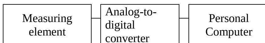
Fig. 2.1. Elements of the information channel
