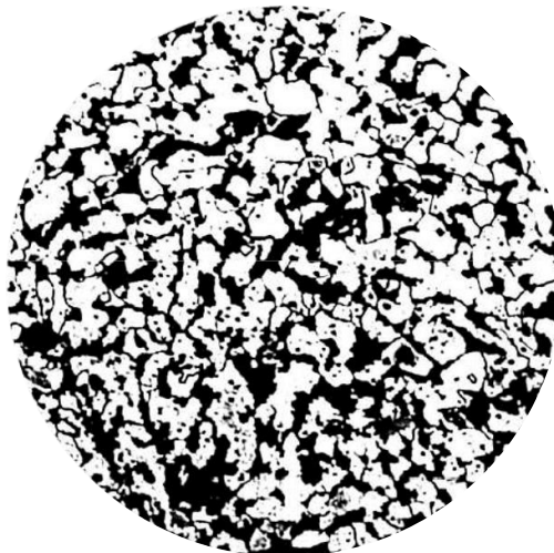
Figure 5.3 – The microstructure of normalization zone
