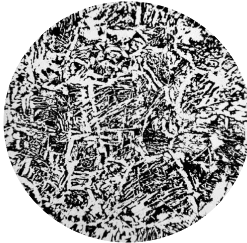
Figure 5.2 – The microstructure of overheated zone
