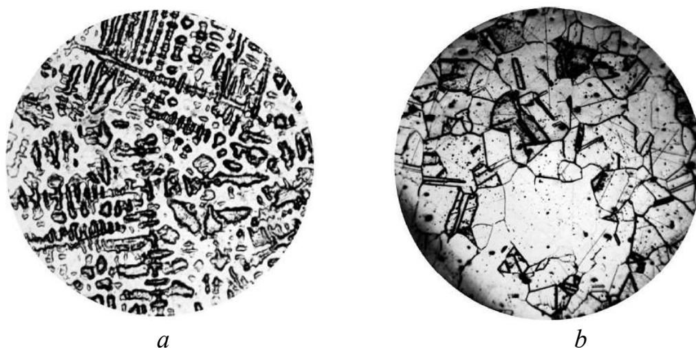
Figure G.1 – Microstructure of single-phase tin cast bronze (6 % Sn) ( a ), after deformation and annealing ( b ), x200
