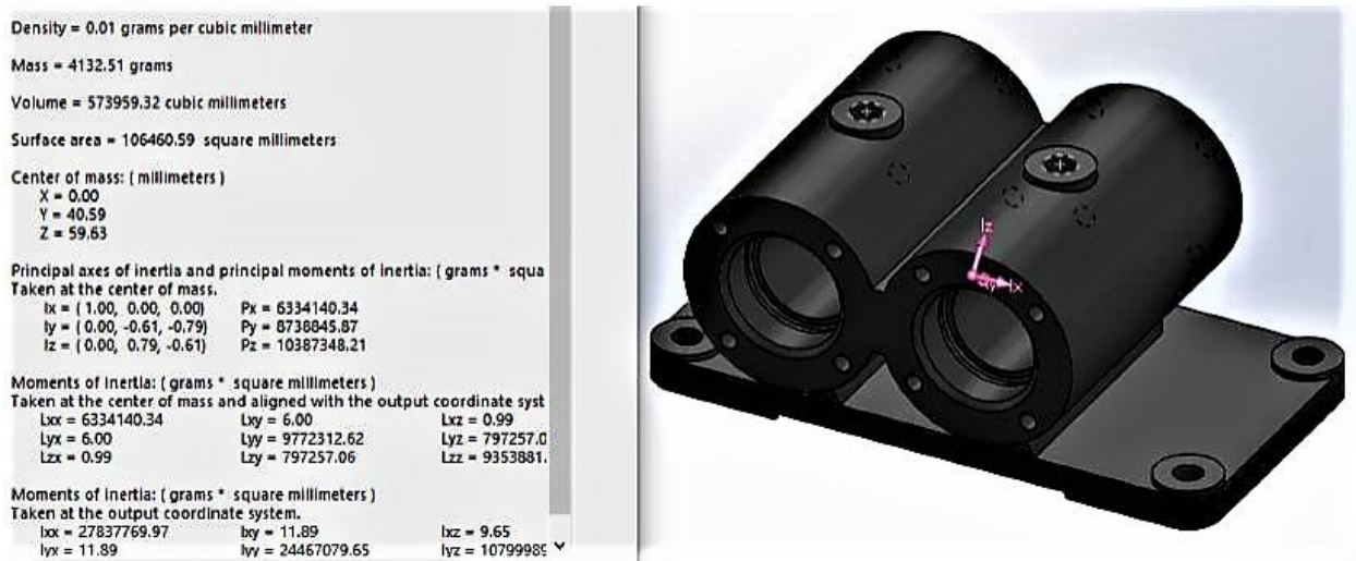
Fig. 1.3 – Characteristics of the part ‘Housing’ and its 3-D model
