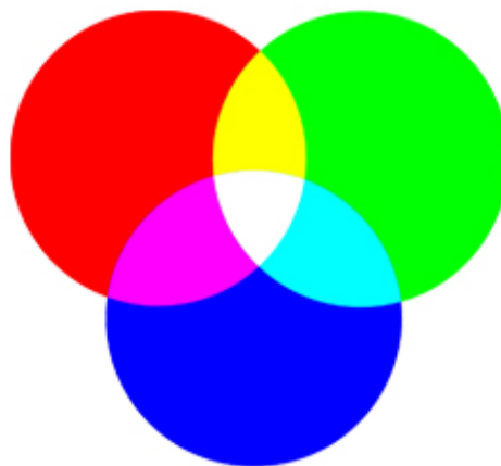
Figure 2.2.1 – The principle of mixing colors in the RGB model
