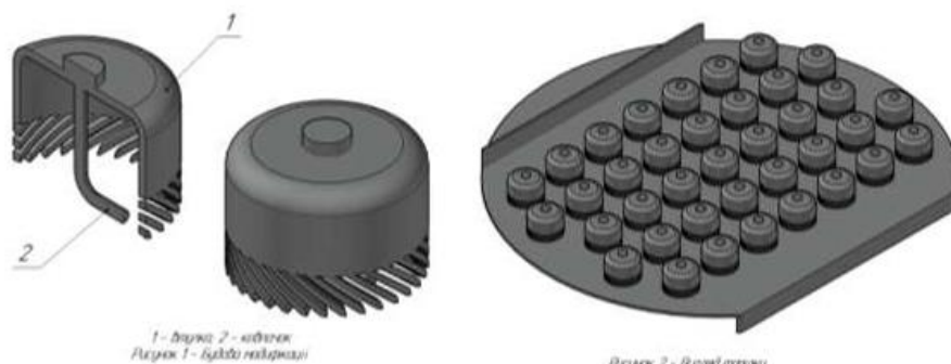
Figure 3 – Visualization of column cap modernization
