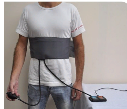
Fig. 2. Applying the belt to record measurement data of respiratory rate
