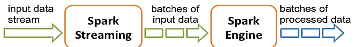
Fig. 7.6. Splitting input data into micro-packets and their further processing
