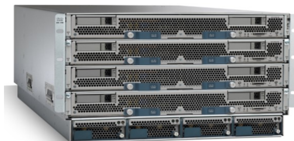
Fig. 3.4. Cisco Unified Computing System 5108
