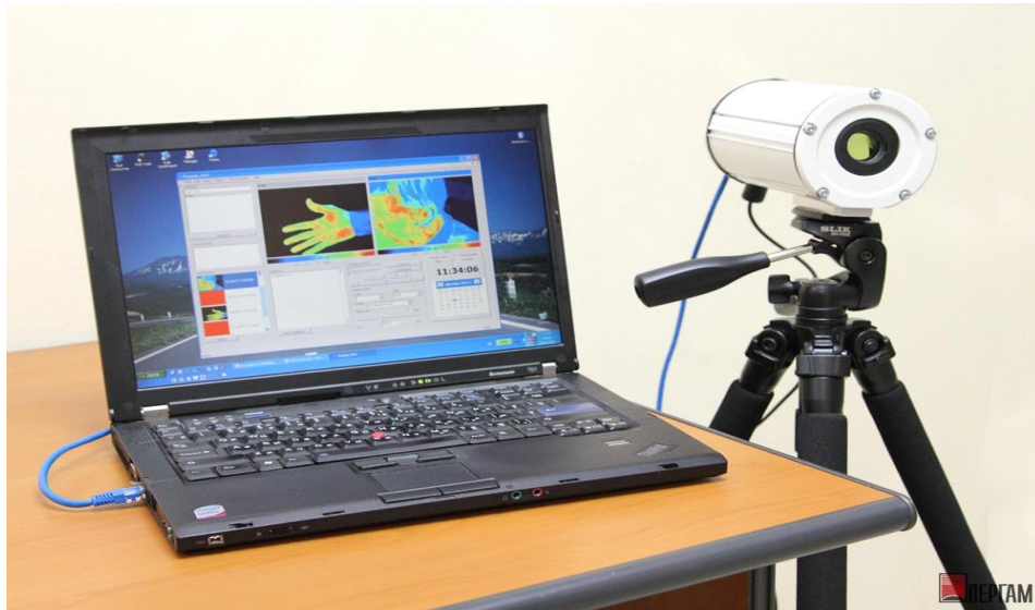
Figure 3.2 – PergaMed thermal imager connected to a computer [16]
