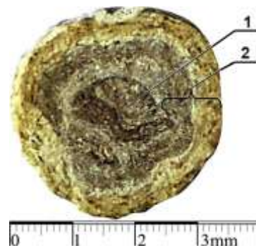
1 – initial center of granulation, 2 – layered structure;
