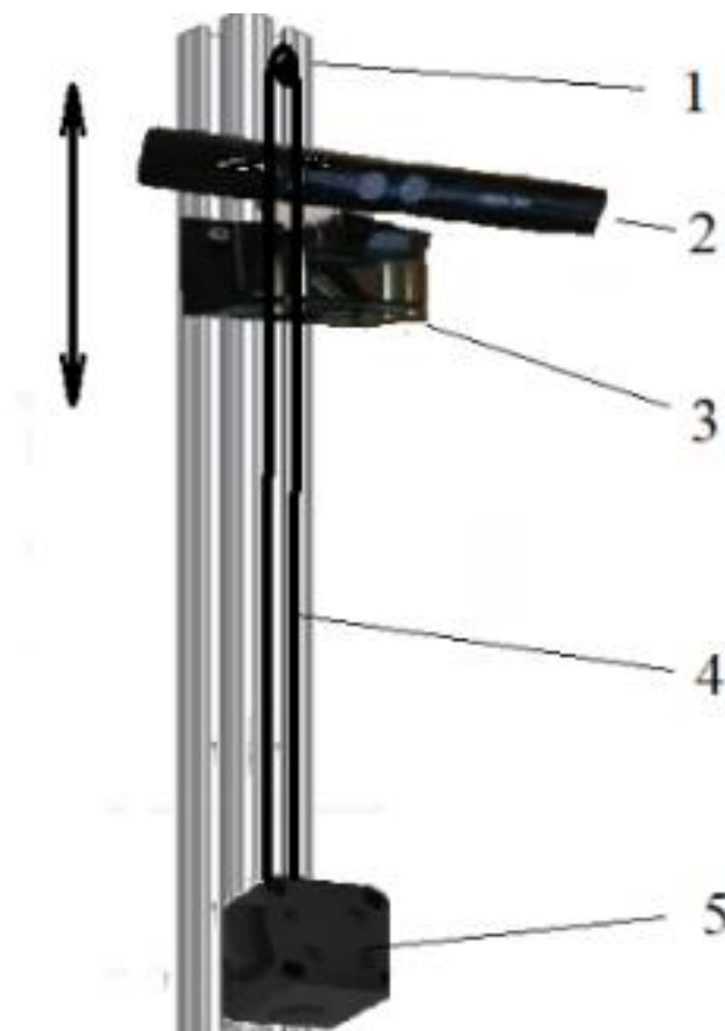
Figure. 2.14 - The main components of the device: 1 - vertical guide from profile 30mm x 30mm; 2 - Kinect v1; 3 – mobile cart on which the camera is located; 4 – belt; 5 - stepper motor.
