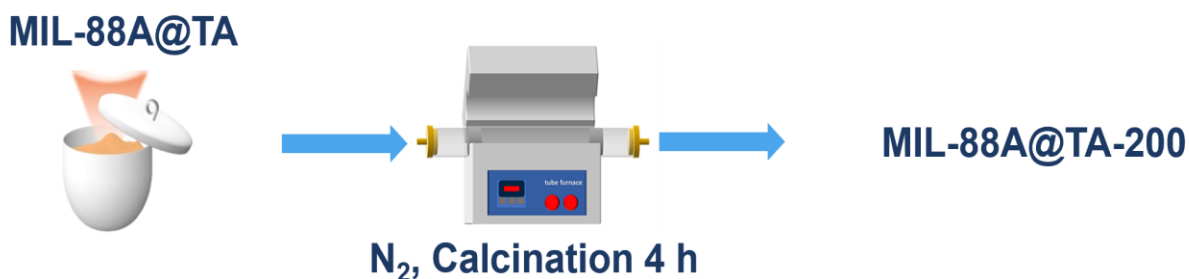
Figure 2.5 Synthesis steps of MIL-88A(Fe)@TA-X.
