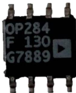
Figure 3.4 - Actual view of the operational amplifier OP284[40]
