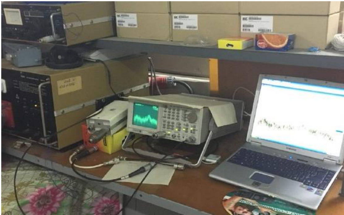
Figure 2.13 - Measuring conductive interference installation
