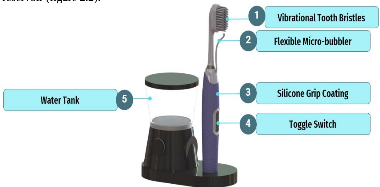
Figure 2.2 – Labelled diagram of the Proposed Sonic Toothbrush
