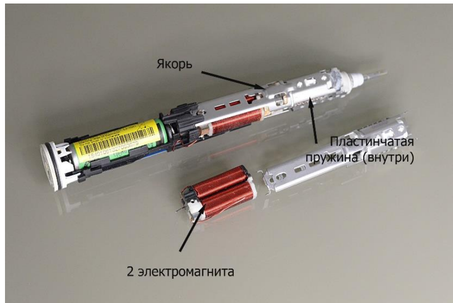
Figure 1.8– Electromagnets inside the product for sound toothbrush
