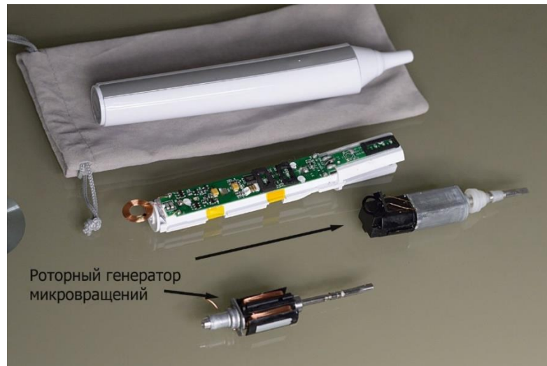
Figure 1.9 – The structure of the sonic toothbrush motor
