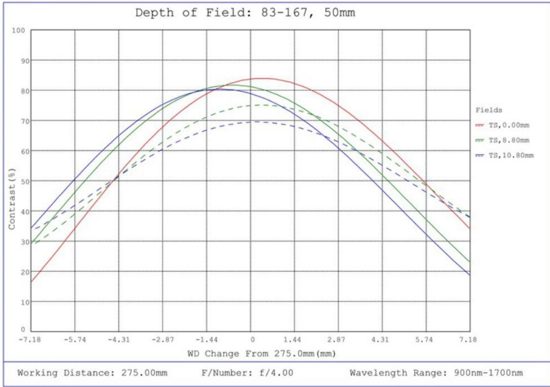
#83-167, 50mm SWIR Series Fixed Focal Length Lens, M42 x 1.0, Depth of Field Plot, 275mm Working Distance, f4
