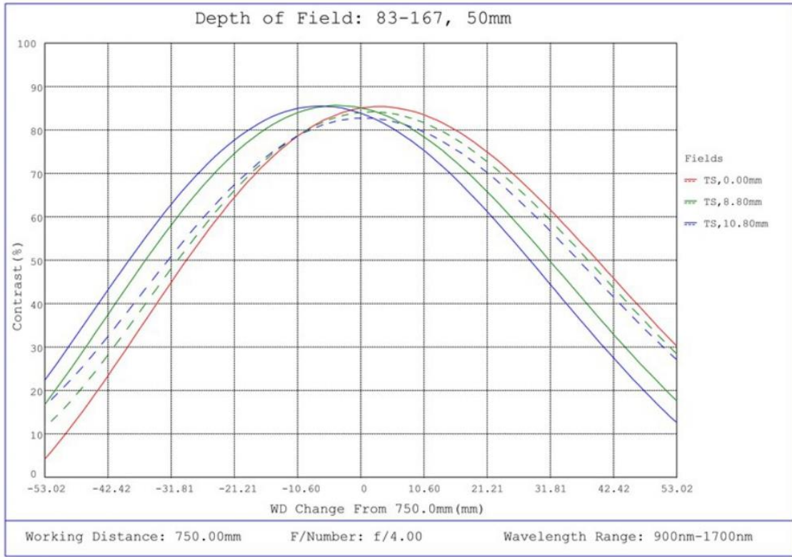
#83-167, 50mm SWIR Series Fixed Focal Length Lens, M42 x 1.0, Depth of Field Plot, 750mm Working Distance, f4
