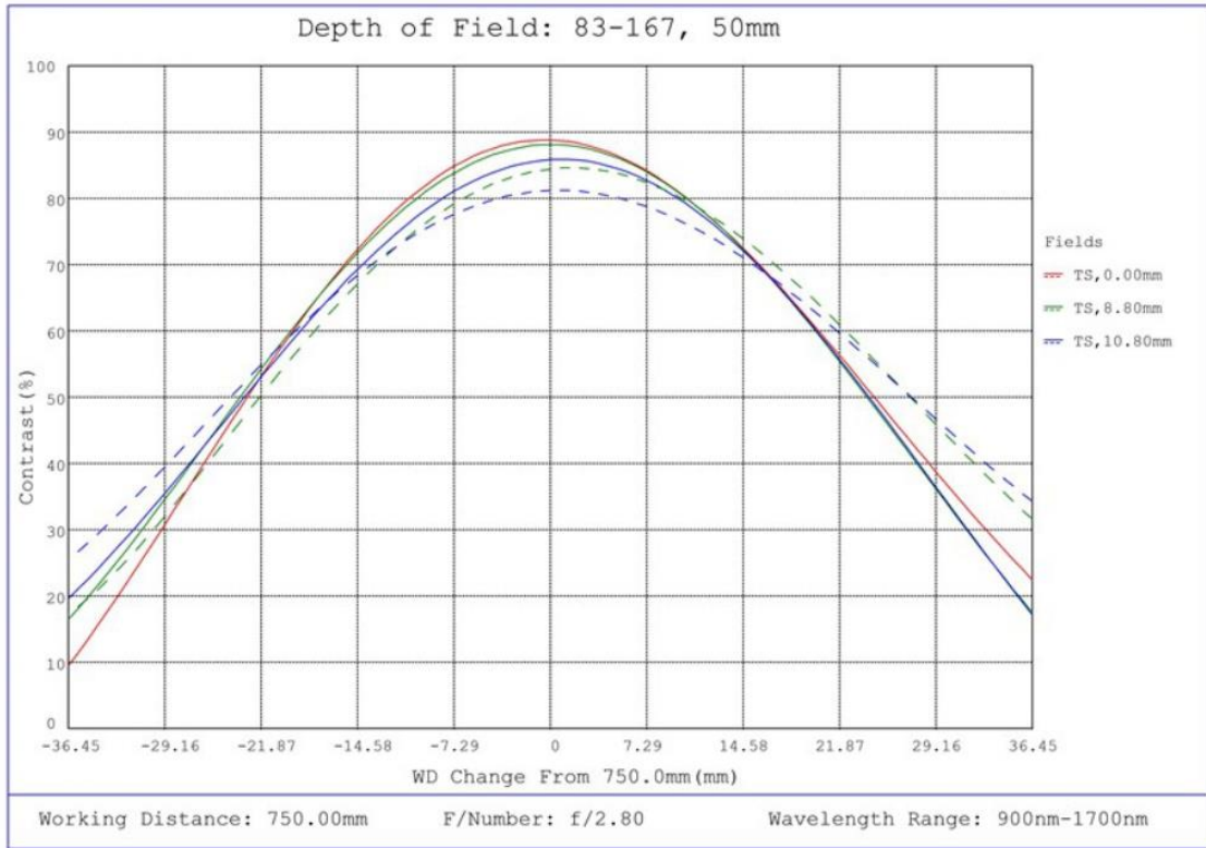
#83-167, 50mm SWIR Series Fixed Focal Length Lens, M42 x 1.0, Depth of Field Plot, 750mm Working Distance, f2.8
