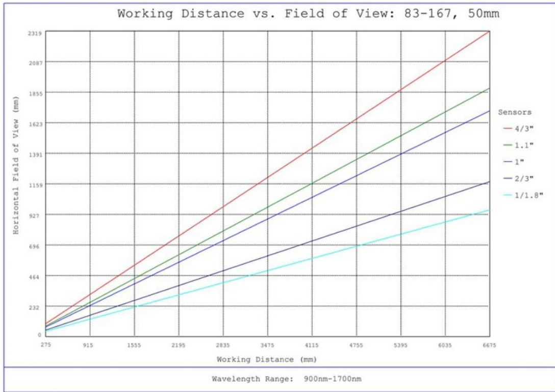
#83-167, 50mm SWIR Series Fixed Focal Length Lens, M42 x 1.0, Working Distance versus Field of View Plot
