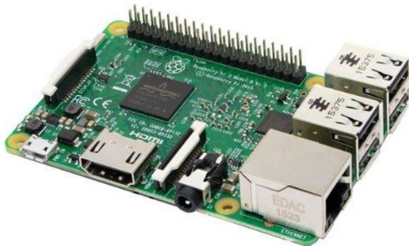
Рис 2.1 Raspberry Pi 3 mod. B, V. 1.2
