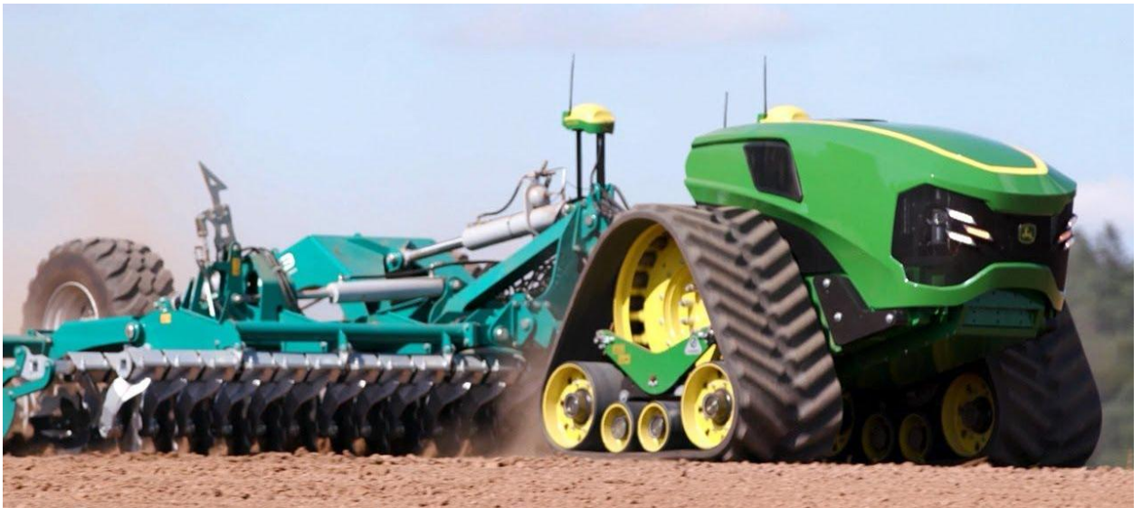
Рисунок 1.8 - Autonomous cab-less tractor, developed by John Deere
