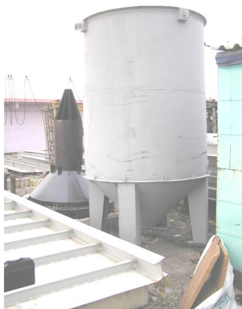
Figure 4.6 – The scheme of vertical sedimentation tank with a central admission tube with a bell
