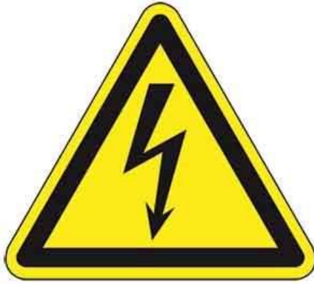
Fig. 2.9. Safety Signal “Caution Electrical Voltage”
