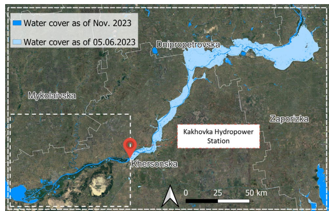
Fig. 2. Comparison of the water cover before the dam damage (June 5, 2023) and after (October 31, 2023).
