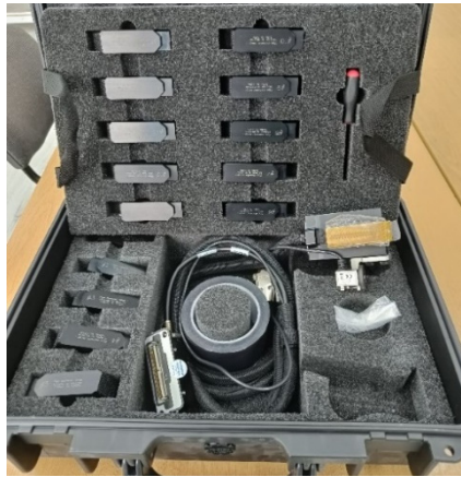
Fig. 6 Set of accessories for OD pipe eddy current inspection using flexible eddy current array probe FBB-051-500-032
