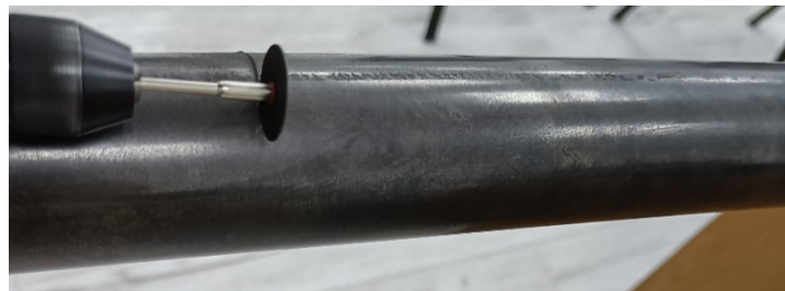
Fig. 3 Fabrication of surface notch type discontinuity using small milling machine
