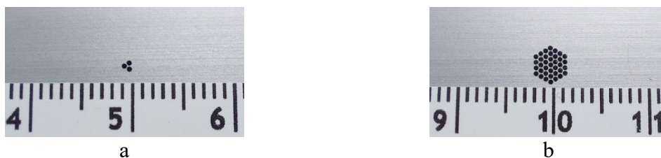
Fig. 3. Circular defects of varying cluster densities in sample (a – defect №10, b – defect №8)
