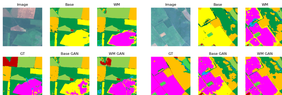
Fig. 2. Visualization of satellite imagery (Image), true segmentation masks (GT), results of base models (Base, Base GAN), and results of models using weight masks (WM, WM GAN).
