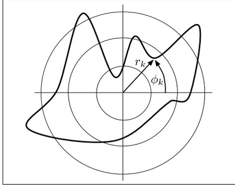
Fig. 1. Sketch of an attractor for a PSS. The dynamics evolves at a constant angular velocity  $\dot{\phi}_k(t) = \omega_k t$  on the black thick curve
